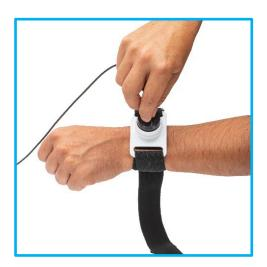
5. Ensure the cable is routed through the cut out in the cap and secure by closing the cap.
