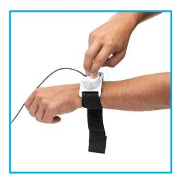
6. The foam mechanism on the cap provides light pressure on the Transducer. It ensures good contact to the gel and skin over the treatment area for proper ultrasound transmission.
